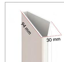
Legs made from 94x30mm pentagon-shaped 2mm steel tube.
