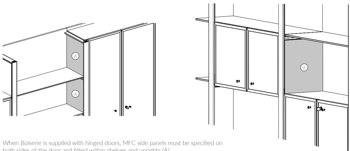
When Boiserie is supplied with hinged doors, MFC side panels must be specified on both sides of the door and fitted within shelves and uprights (A).
